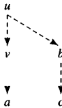
FIG. 7.19 For v and w to satisfy Dfn(v) \leq Dfn(w) , w may be in any of the positions of v , a , b , or c , where b is some descendant of u visited after all the tree descendants of v . A dotted arrow represents a possibly empty path, and a dashed arrow represents a non-empty path.
